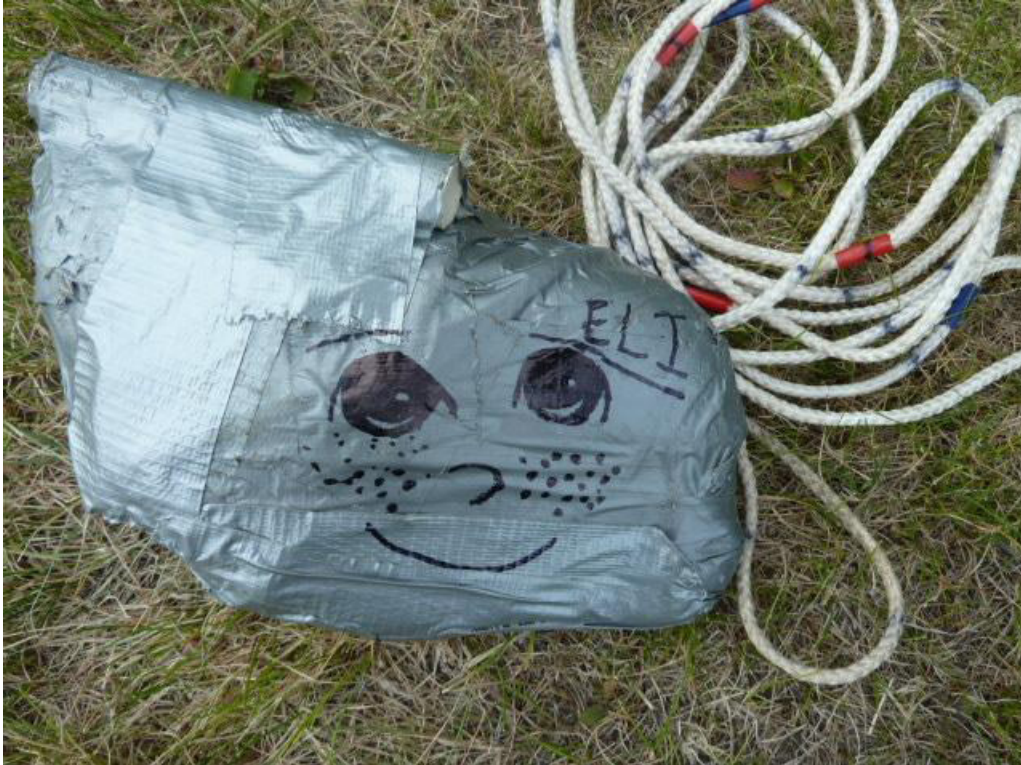
Depth measurement rock on a string, developed and photographed by Kendall, Cassandra, and Bonnie.
