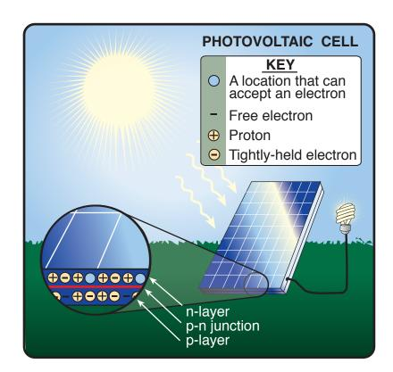
A **photovoltaic (PV) solar cell** is a device that converts the radiant energy (carried by the sun's heat and light) into electricity.
