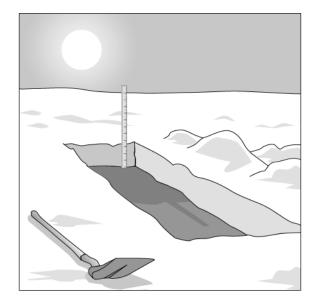
Place the meterstick along face of the snow wall. Make sure the zero end of the stick is sitting on the ground.
