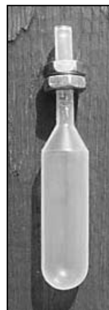
The plastic eye dropper above has been weighted with two brass nuts to provide the added weight needed to sink the Cartesian diver.
