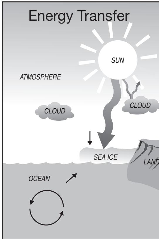
2. The ocean warms the ice through conduction. The atmosphere warms the ocean through conduction. The sun warms the ocean and the ice through radiation. The ocean redistributes energy within itself by convection.
