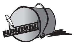
Step 3:Mark this line and label it at one-inch intervals, starting from the bottom.
